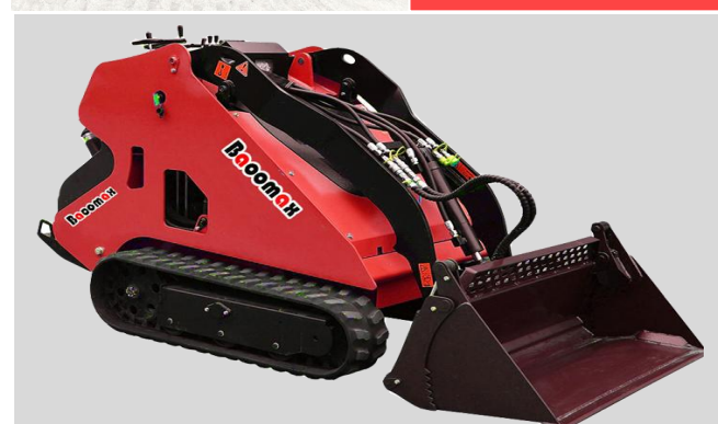
BA2T mini track skid steer loader(Baomax) Engine :25HP Kubota diesel Loading capacity: 450KG Rubber track:200x72x39 Machine width:1103mm
