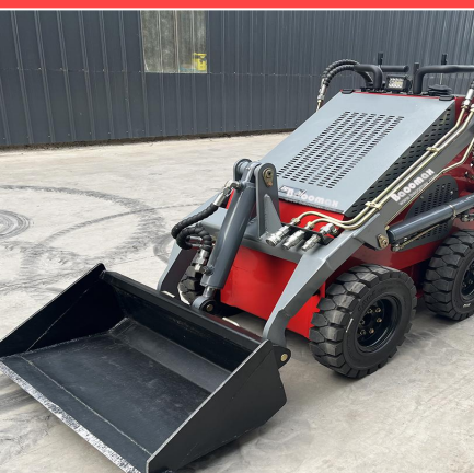
BA30 mini skid steer loader (Baomax) Engine : 23HP USA Briggs&Stratton Loading capacity: 380KG Wheel tires :20*10-10 Machine width:1150mm Tire model :20x10-10
