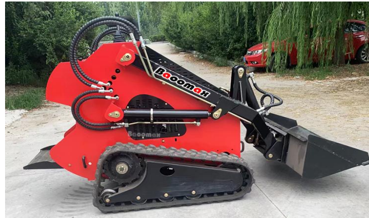
BA30T mini track loader (Baomax) Engine : 23HP USA Briggs&Stratton Loading capacity: 380KG Rubber track :180x36x72 Machine width:980mm Track model :180x36x72
